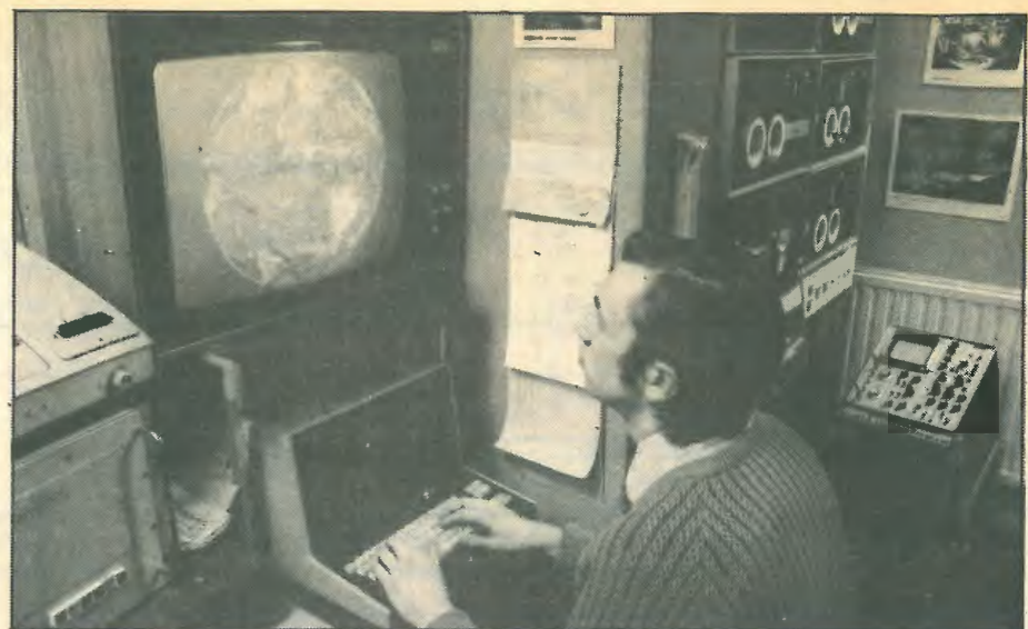
One of eight registered primary data users, Mike Christieson, at his station. From left to right are colour-display electronics, computer-terminal and v.d.u. with colour monitor above it showing p.d.u.s. full-disc image, and the PDP9 mini-computer with four tape drives. The white panel below the tape drives is the satellite interface.
